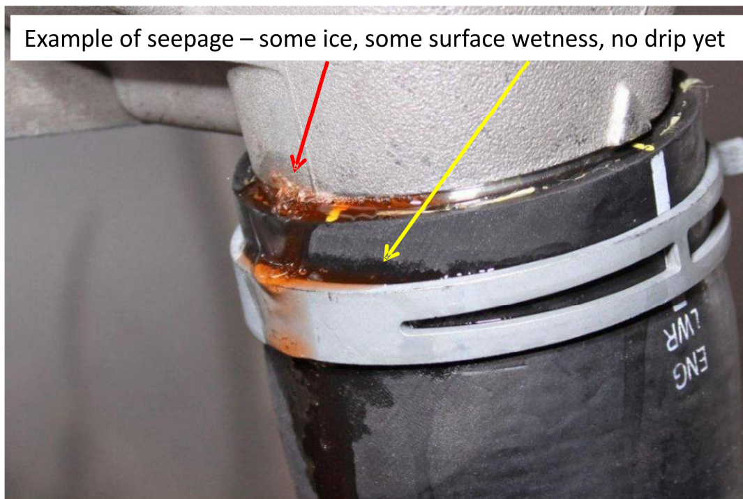
Figure E1: Example of Seepage
